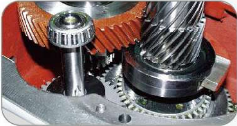
Strong back gear transmission instead of timing belt for Hi-Low speed
