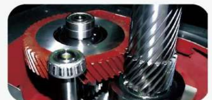
Strong back gear transmitting instead of timing belt for Hi-Low speed
