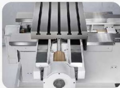
Box way design on all slideways
