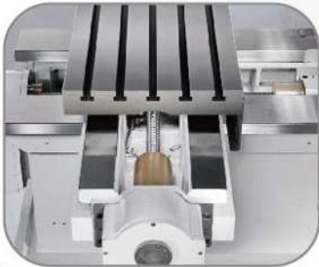
Box way design on all slideways
