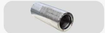
Large quill diameter 110mm (4.33") material S45C(SAE1045) with high-frequency induction hardening and chrome plated
