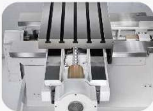
Box way design on all slideways.
