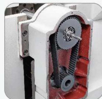
1:2 ratio timing belt pulleys on XYZ axes increase drive torque, and reduce the cost for axes motors.
