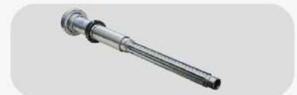
NST#40 spindle material SCM415 (SAE4115) fully hardened and precise ground
