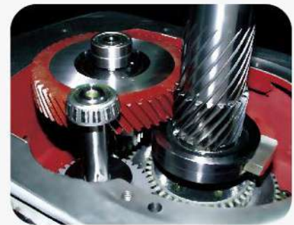
5HP heavy cutting milling head transmitted by gears
