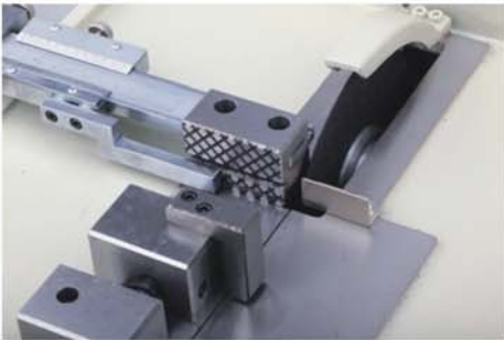
V shape clamping for round workpiece
