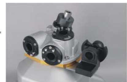
Grinding the relief angle
