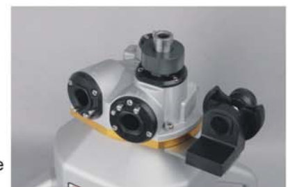
Grinding the end mill pitch
