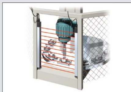
Installing light curtains in an upside-down orientation may be necessary to shift the dead zone position
