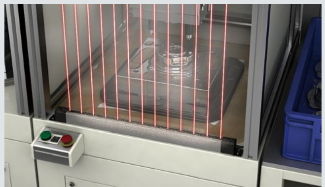
The bottom part of the vertical installation may be damaged by or may malfunction due to the dirt or liquids in the air.
